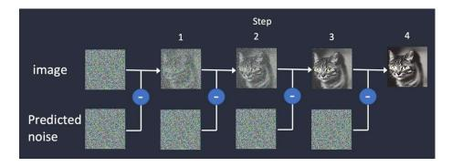
90. In sum, diffusion is a way for a machine-learning model to calculate how to reconstruct a copy of its training images. For each training image, a diffusion model finds the sequence of denoising steps to reconstruct that specific image. Then it stores this sequence of steps. In practice, this training would be repeated for many images—likely millions or billions. A diffusion
